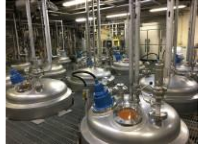
Beer fermentation tanks Pilot Plant (Kanagawa Prefecture)
