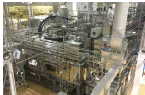
Air rinse facility introduced at the Shonan Plant
