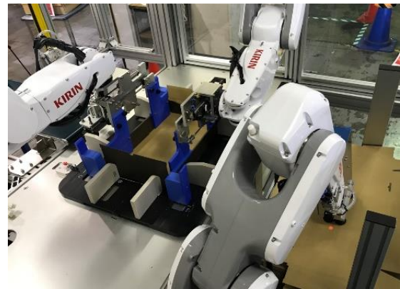
Forming of inner box by new robot
