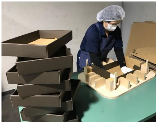
Conventional inner box forming work by hand
